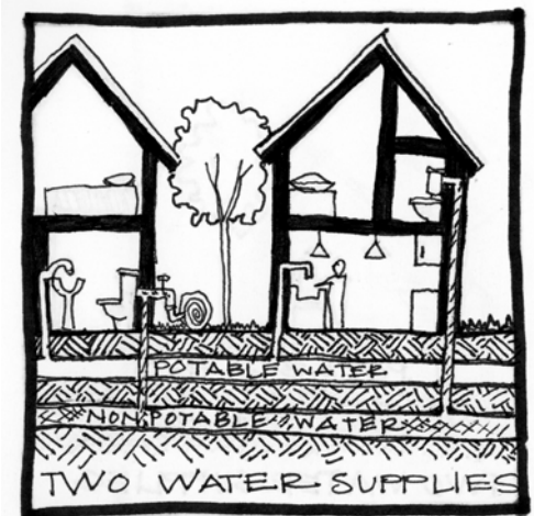
Figure 55: To maximize benefits of any future water recycling plant, two sets of water supply pipes should be built.
