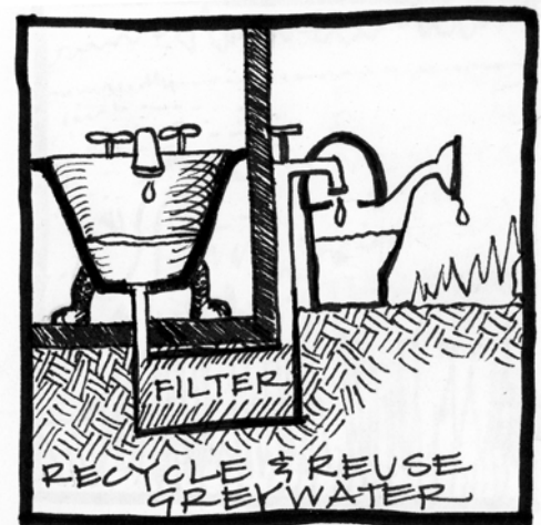
Figure 53: Greywater can be recycled and reused in many small ways.
