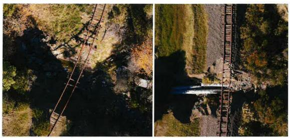
Aerial Ph: MP 129.67 Erosion of 3-span Timber Trestle
