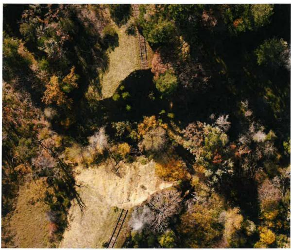
Aerial Ph: MP 125 Baker Creek Washout & Erosion 160' long by 35' deep from unmaintained & undersized culvert
