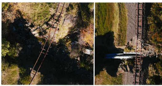
Aerial Ph: MP 129.67 Erosion of 3-span Timber Trestle
