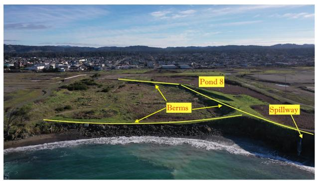
Photo 1 (with Graphics): Looking east toward downtown Fort Bragg, this aerial shot of OE-E shows that, for the time being, the ponds in this section of the old mill site, are contained by the rocks and dirt used to create the berms holding the sediments from entering the bay referred to historically as Soldier Harbor.
